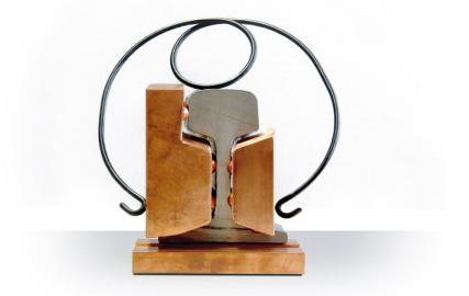
The electrode is introduced vertically from above into the welding gap. During welding the electrode is weaved, reaching both sides of the rail flanks, its stops for a short time. If the weld pool overheats during welding, welding must be interrupted for some time. We recommend checking the amperage and reduce it if necessary.
