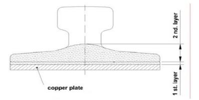
Reaching both sides of the rail flanks, the electrode should be stopped for a short time to obtain a perfect penetration.
