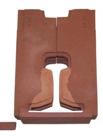
Preheating of the joint faces by external means of fuel oxygen flame is usually required to assure elimination of all moisture in the mould and raise the rail parent material to promote complete fusion. After the weld metal is solid and cooled down, the mould is removed and the joint is finished by grinding.
